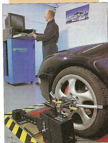
For maximum accuracy, infra-red cameras attached to wheel centres, not rims or tyres
