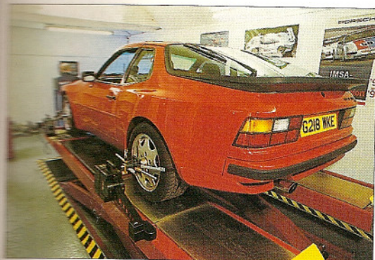
Beissbarth system features lift to allow access beneath car; 944S2 showed some measurements beyond specified limits
